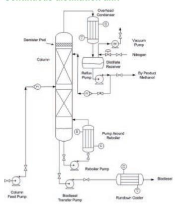
not like to be started up and shutdown. The unsteady state conditions that occur may cause off spec product to be produced. On startup a continuous column may not produce on spec product until the column lines out (reaches steady state).
